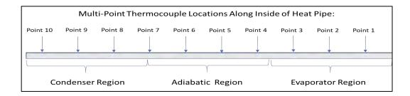
The ACT heat pipe has an internal thermowell running down the center of the heat pipe. A multi-point thermocouple is inserted into the heat pipe.
