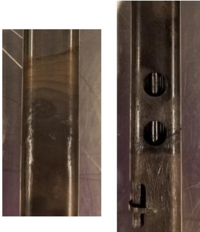
Figure 13. Images of the triple bubbler shroud showing the effects of salt climbing the shroud. Figure reproduced courtesy of Williams, A., Galbreth, G. and Sanders, J., MPACT Working Group Meeting, April 2019.
