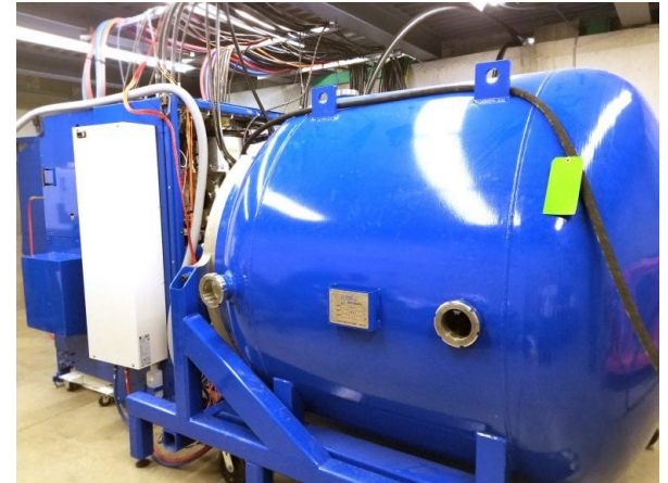
Phoenix high yield D-T neutron generator
