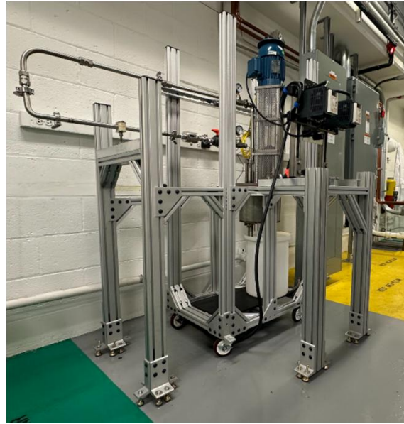
Figure 12. (left) P&ID and (right) image of water testing loop
