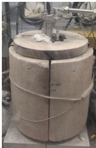
Figure 7. Photo of salt purification system using uranium metal feedstock. Fabrication of the salt purification system was funded by DOE NE-5's Advanced Reactor Safeguards and Security program
