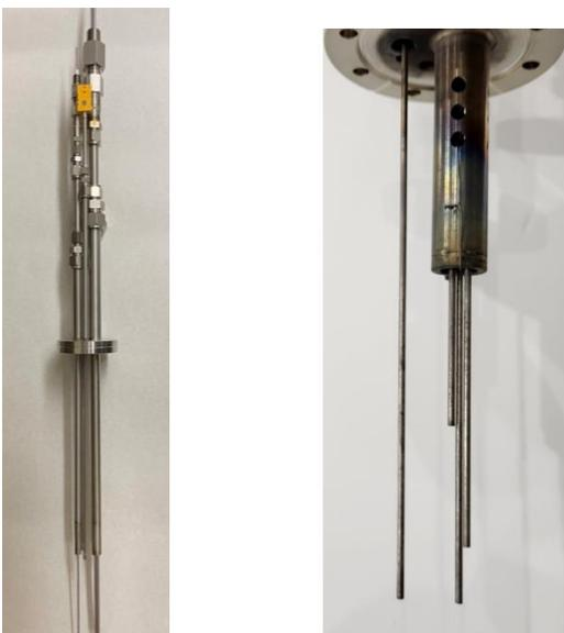
**Figure 15.** Photos of the electrochemical sensor assembly (*left*) before deployment in FASTR loop, and (*right*) after operation in FASTR.
