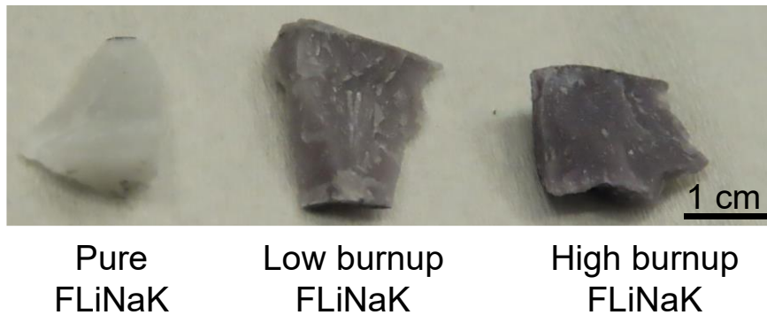
Figure 1: Frozen samples of synthesized pure, low burnup, and high burnup FLiNaK
