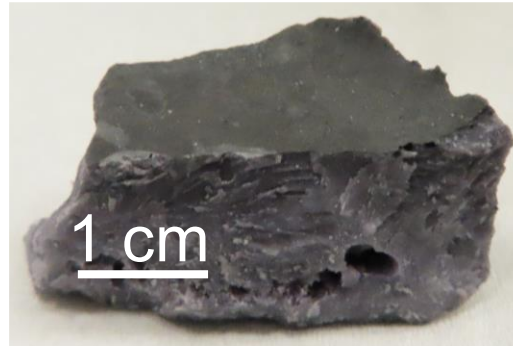
Figure 8: Cross-section of frozen salt that shows graphite particles at salt surface.
