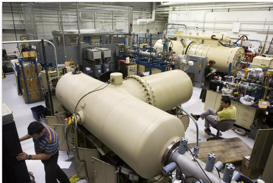
Materials—To support our wide range of materials research (Was) there are two facilities: the Michigan Ion Beam Laboratory (MIBL) and the Irradiated Materials Testing Laboratory (IMTL). The MIBL is the only triple ion beam facility in the US and also includes the capability to conduct dual ion
