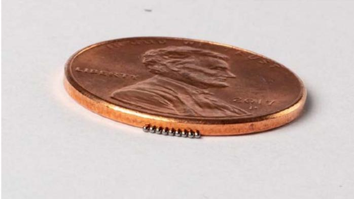
The ORNL-designed MiniFuel significantly decreases the size of fuel specimens and capsules that are irradiated in ORNL's High Flux Isotope Reactor. The smaller experiments allow researchers to better control various conditions during irradiation and improve interpretation of data during post-irradiation examination.
