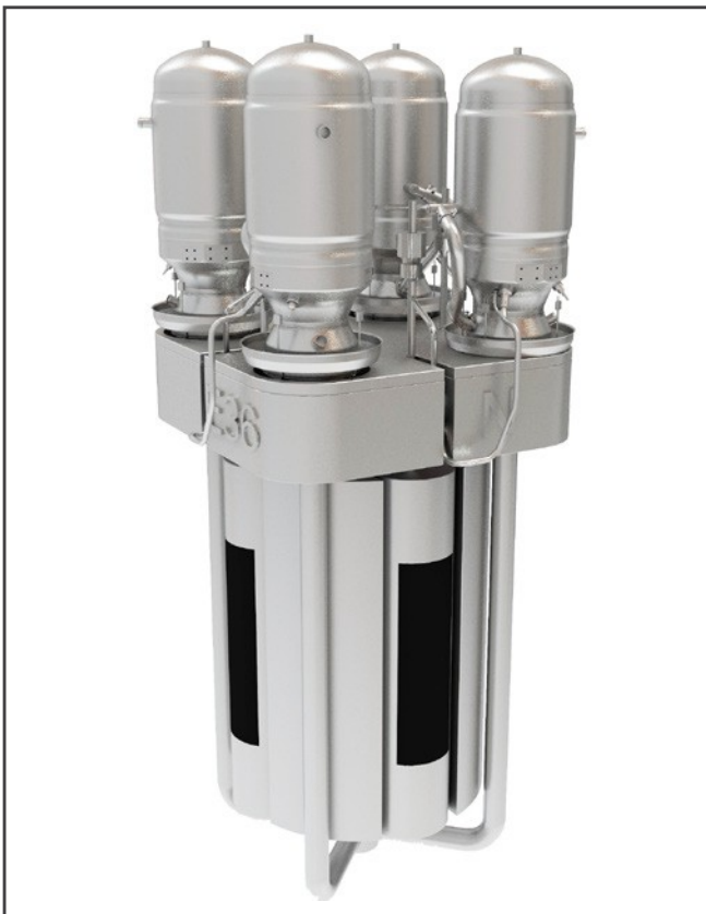
MARVEL reactor concept with Stirling engines.
