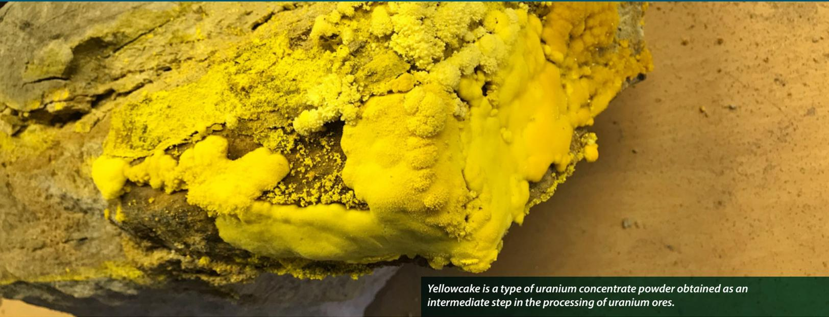
*Yellowcake is a type of uranium concentrate powder obtained as an intermediate step in the processing of uranium ores.*
