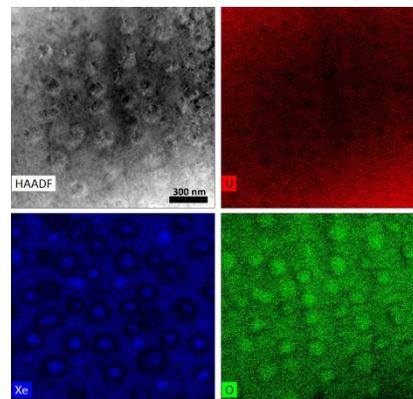
**Stem-EDS images showing circular features in Xe-implanted UO<sub>2</sub>**
