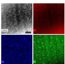
Stem-EDS images showing circular features in Xe-implanted UO<sub>2</sub>
