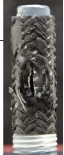
Time [ms] Example test to failure with SiC-f/SiC-m
