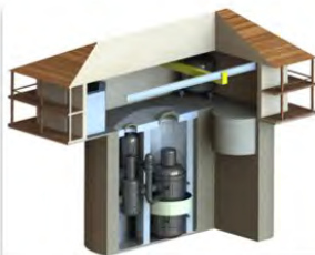
The FMR Reactor System
