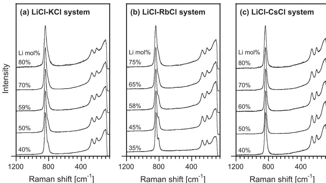
**Figure 2-4.** Raman spectra of alkali chlorides including 3 mol% U(VI) at 823 K. (a) LiCl-KCl system. (b) LiCl-RbCl system. (c) LiCl-CsCl system. From Fujii et al.<sup>27</sup>
