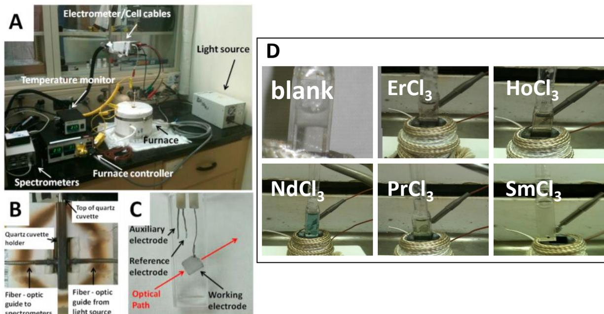
**Figure 2-7.** The spectroelectrochemistry setup design, relying on UV-vis absorbance spectroscopy (A), with a picture of the cross section of the furnace/cell holder (B), and molten salt cell with electrodes in place (C), along with pictures of melts containing lanthanides (D). From Schroll et al.<sup>5</sup>
