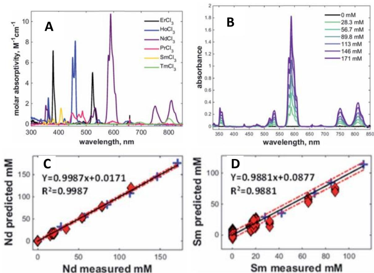
**Figure 2-2.** (A) UV-vis absorbance fingerprints of 6 lanthanides within LiCl-KCl eutectic and example (B) of how UV-vis fingerprints vary with lanthanide concentration within the salt melt. These data were used to build chemometric models to quantify the lanthanides in the melt where the resulting parity plots are shown for two lanthanides, (C) Nd and (D) Sm. From Scroll et al.<sup>3</sup>
