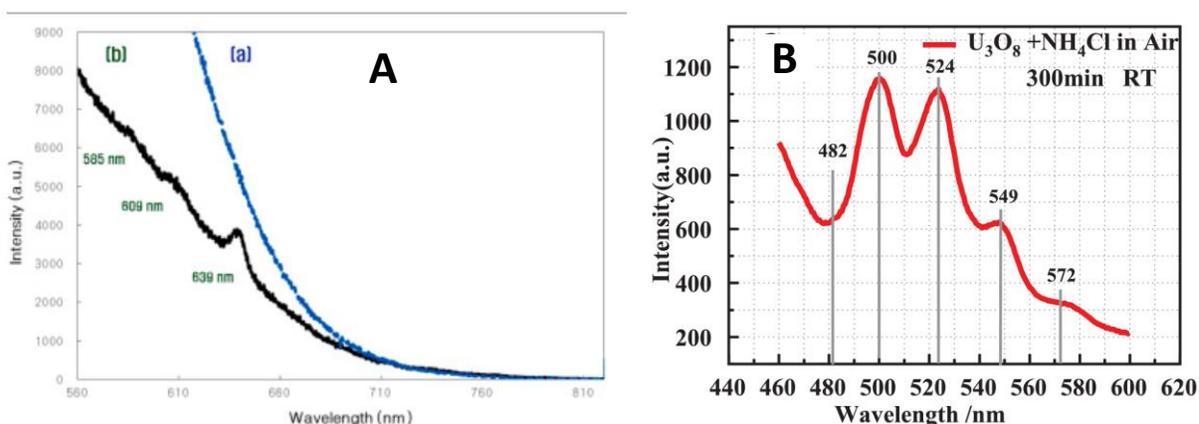
**Figure 2-5.** Fluorescence spectra of (A)  $\text{UCl}_3$  in LiCl eutectic melt (black line) mixed in HmCl (1-hexyl-3-methyl-imidazolium chloride) ionic liquid ( $\lambda_{\text{ex}}=504$  nm) from Im et al.<sup>28</sup>; and (B) dissolved  $\text{U}_3\text{O}_8$  in a quenched LiCl-KCl eutectic in the presence of  $\text{NH}_4\text{Cl}$ . The concentration of U in the quenched salt was 0.47 wt. %. From Liu et al.<sup>29</sup>
