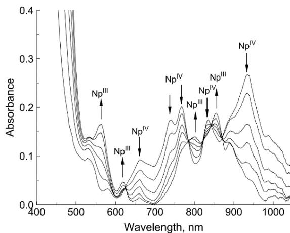
**Figure 2-6.** Spectra recorded during electrochemical reduction of  $\text{Np(IV)}$  to  $\text{Np(III)}$  in 3LiCl-2KCl eutectic melt at 450 °C. Initial concentration of neptunium(IV) - ca. 0.015 mol/L. Total time of reduction - 1280 sec, current - 5 mA. From Polovov et al.<sup>36</sup>
