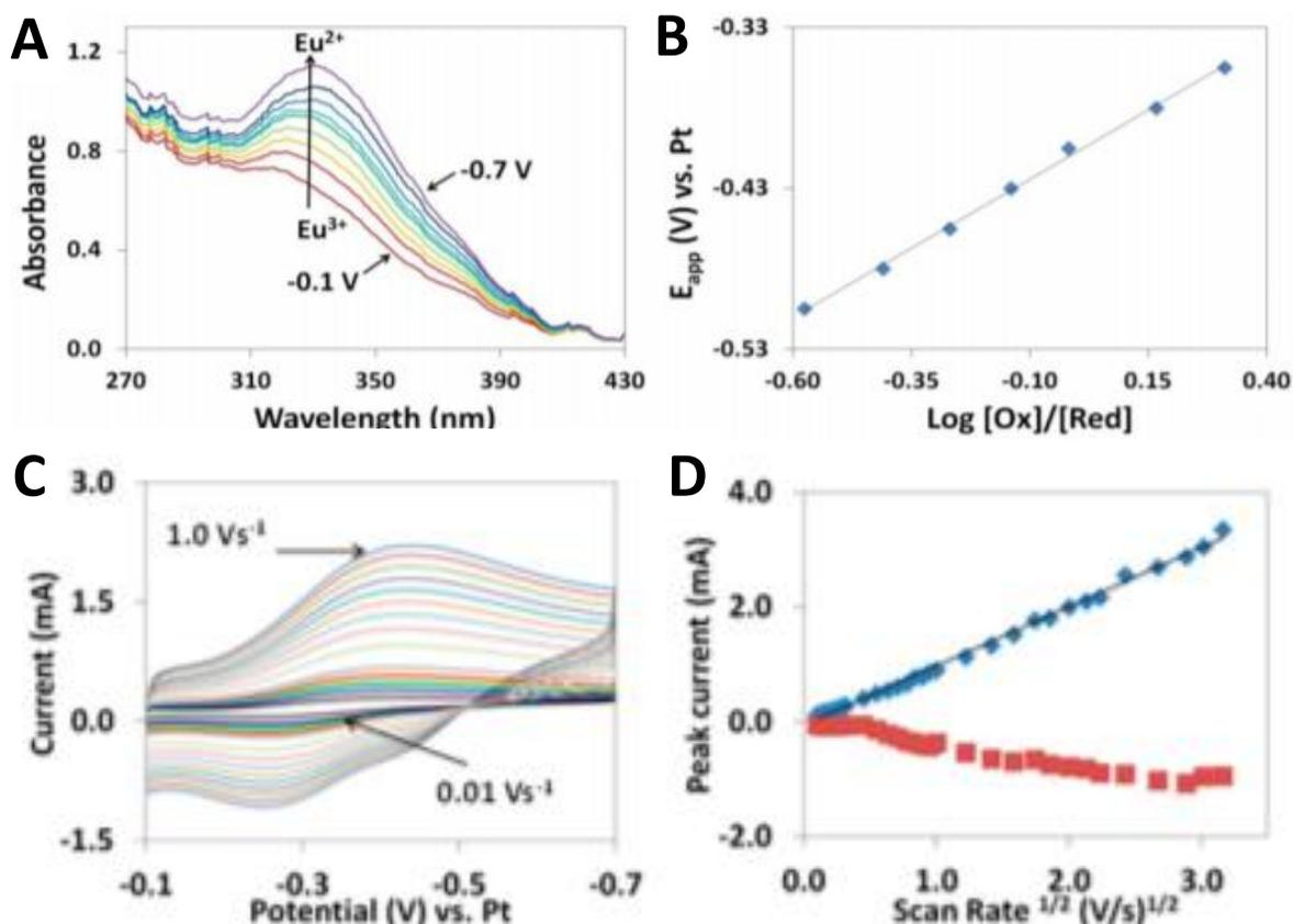
**Figure 2-1.** (A,B) Figure demonstrating the use of spectroelectrochemistry to characterize the formal reduction potential and optical fingerprints of Eu in chloride based eutectic<sup>4</sup>; (C,D) Figure demonstrating use of spectroelectrochemistry to calculate diffusion coefficients of Eu in chloride based eutectic. From Schroll et al.<sup>5</sup>
