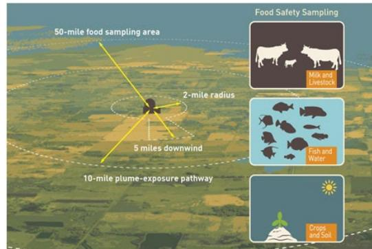
Note: A 2-mile ring around the plant is identified for evacuation, along with a 5-mile zone downwind of the projected release path.
