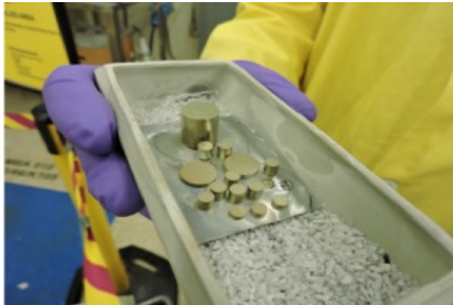
Figure 3. 40%U-ZrH x pellets fabricated by powder metallurgy. Samples were fabricated in dimensions required for thermophysical property measurements.
