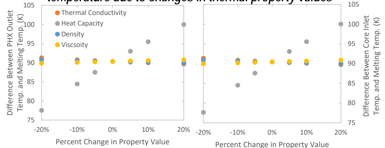
Difference between out temperatures and nominal melting temperature due to changes in thermal property values
