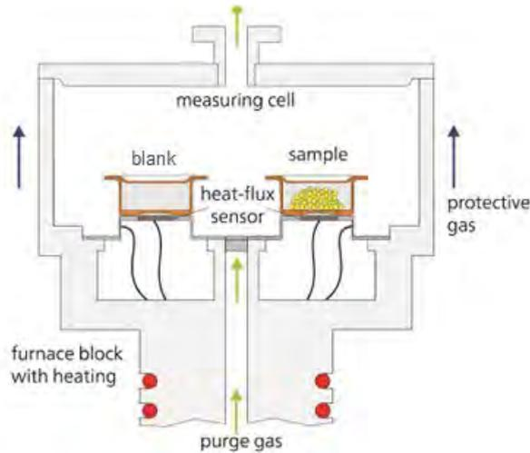
Ramp temperature at constant rate and measure difference in heat flow through salt sample and empty crucible
