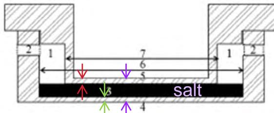
Schematic diagram of the crucible for measuring thermal diffusivity: 1-space for expansion; 2- holes for gas to escape; 3- molten salt; 4-crucible bottom; 5-lid bottom; 6-inner diameter; 7- inferior diameter.
