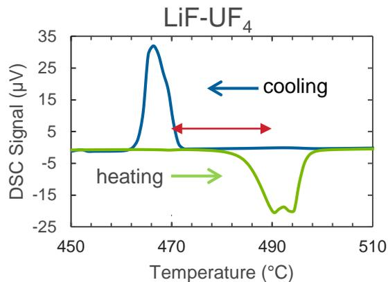
Significant super cooling can occur, so only use heating data
