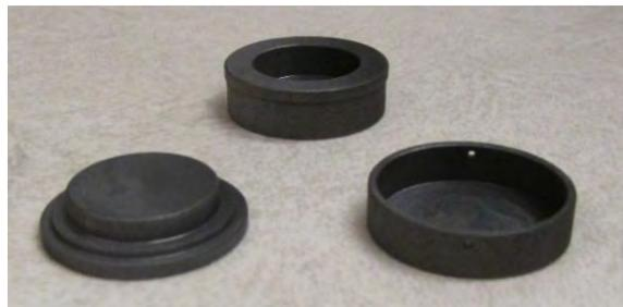
Graphite LFA Cells: closed (top) and open with the lid inverted (bottom left) and the crucible (left).
