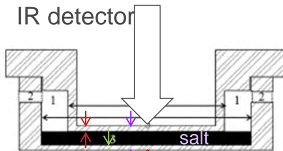
Schematic diagram of the crucible for measuring thermal diffusivity: 1-spacing for expansion; 2- holes for gas to escape; 3- molten salt; 4-crucible bottom; 5-lid bottom; 6-inner diameter of crucible; inferior diameter.
