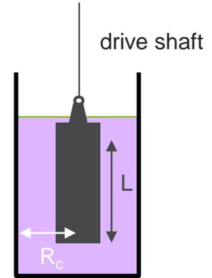
Side view spindle in crucible
