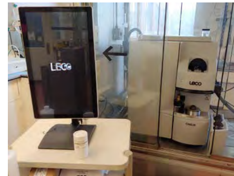
Measurement of oxide concentration in molten salts including beryllium salts by a LECO inert gas fusion analyzer
