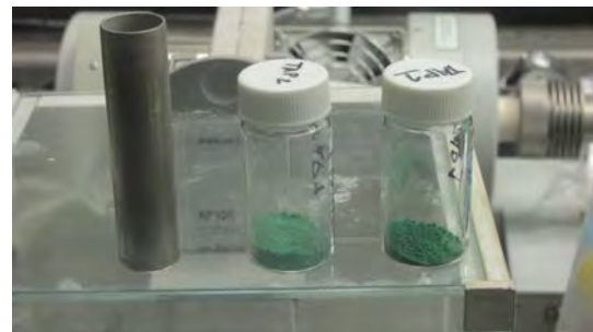
Photo of LiF-UF_4 Mixtures Prior To (left) and After (right) Fusing
