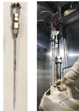
Argonne multielectrode sensor integrated into molten salt loop at ORNL for concentrating solar power applications
