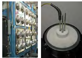
BeF 2 compatible test cell for electrochemical measurements of fundamental fluoride properties
