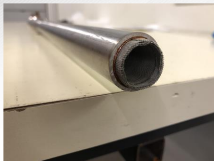
Multi-layered composite screen wick mesh was fabricated (Water as a working fluid).
