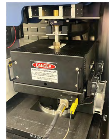
High temperature enclosure
