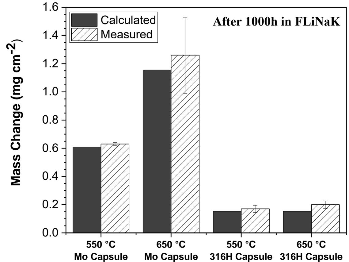
➤ Saturation limits for Fe and Cr are attained after 48 and 125h respectively for the tests in 316H capsules
