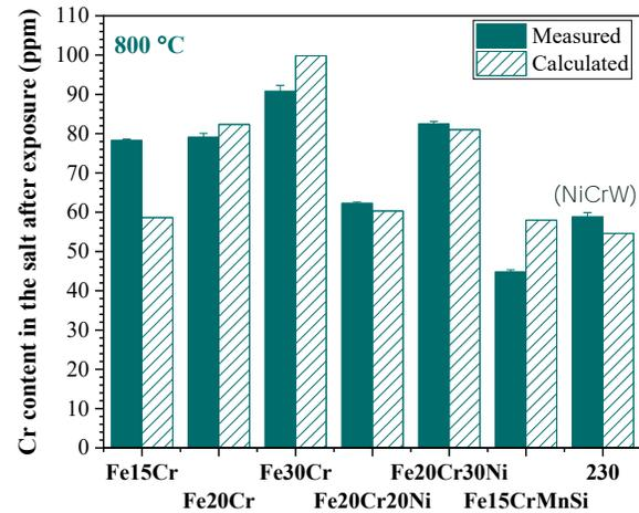
Modeling approach allows predicting dissolution of key phases
