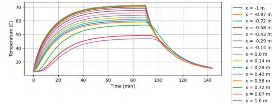
(b) Results Obtained by the Heat Conduction Calculations.
