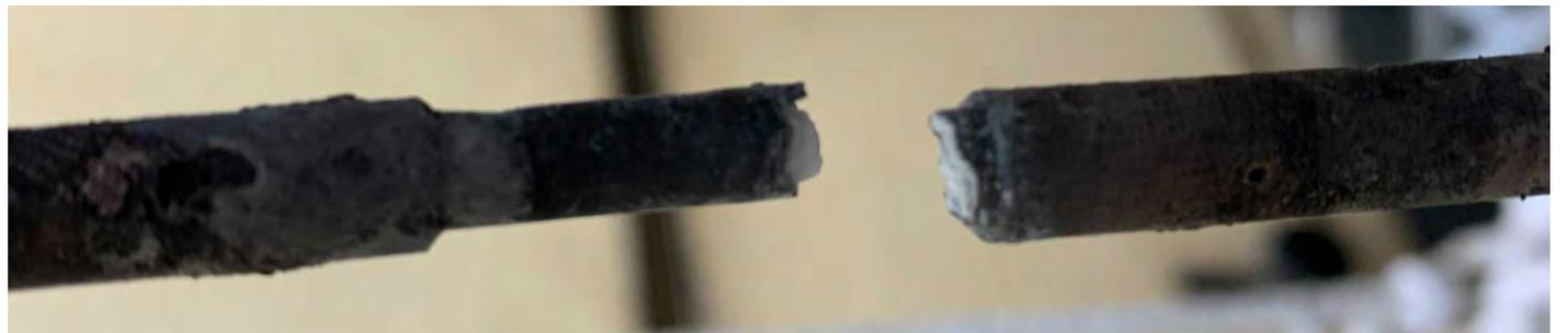
*Irradiated tube failure after about 880 hours*
