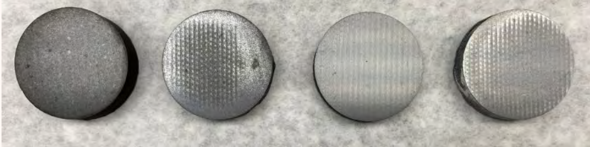
SPS B 4 C disks from lowest density produced, left, to highest density, right.
