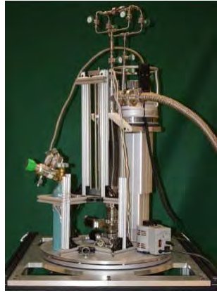
Mass Produced High Purity Heat Pipe Fill And Seal
