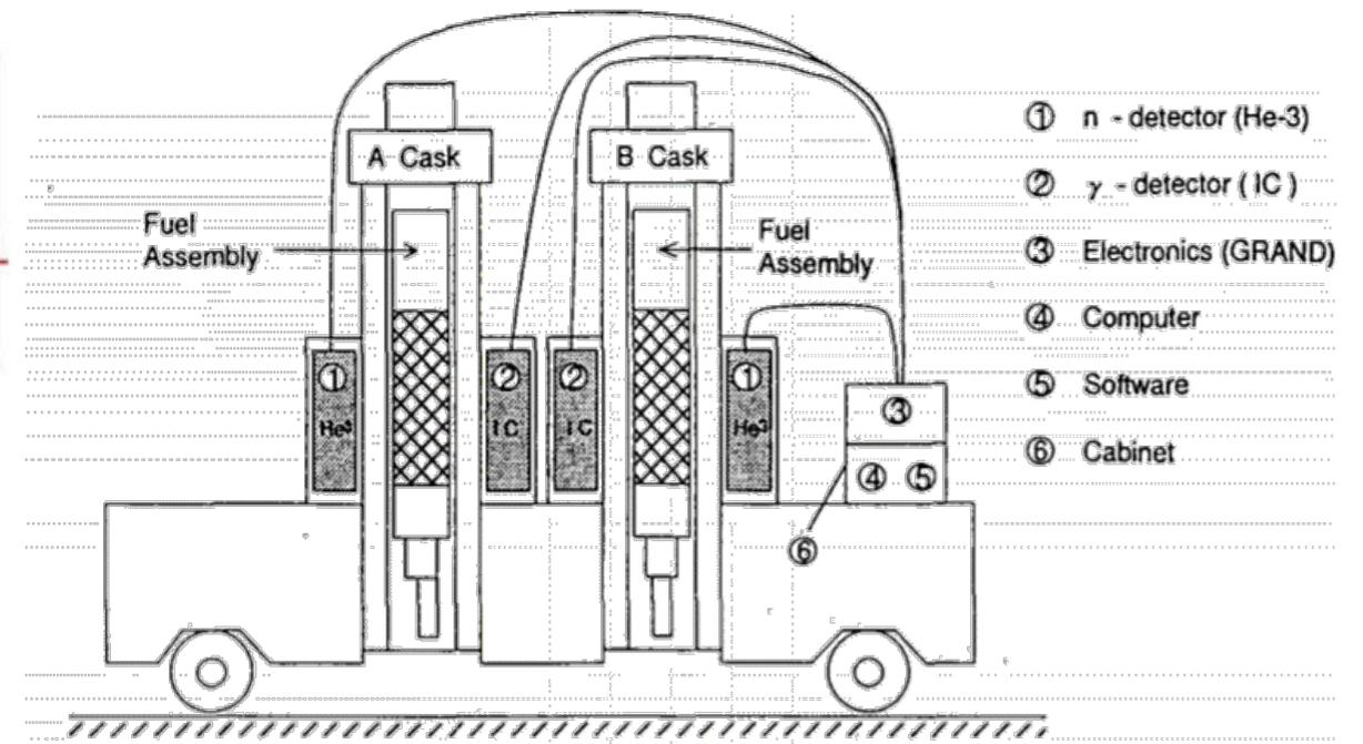
*Ex-Vessel Transfer Machine (EVTM) with instruments*
