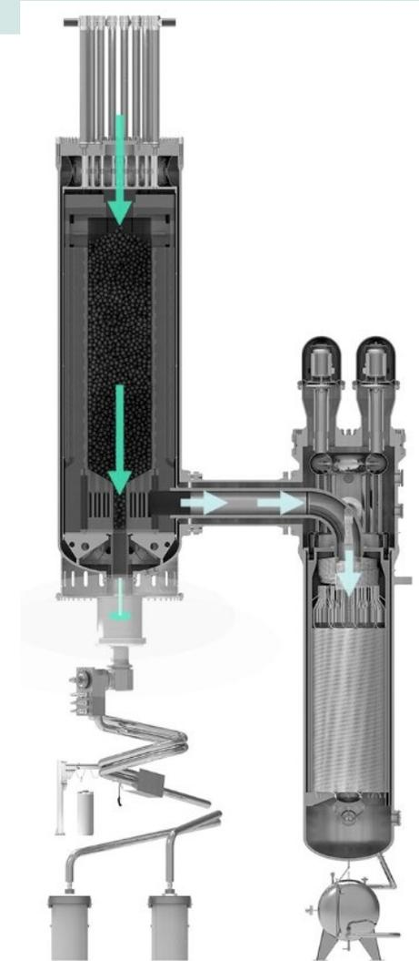
XE-100 Reactor Schematic
