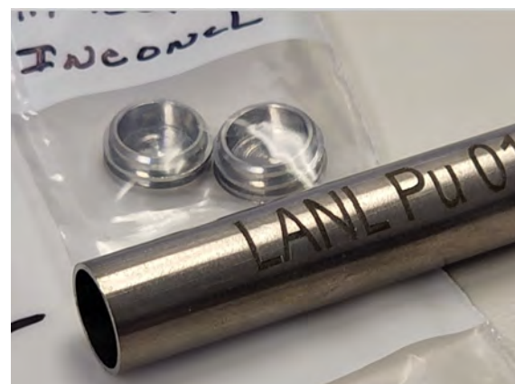
One of the fabricated capsules for shipping pelletized PuCl 3 -NaCl eutectic from INL to LANL.
