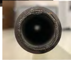
Multi-layered composite screen wick mesh was fabricated.
