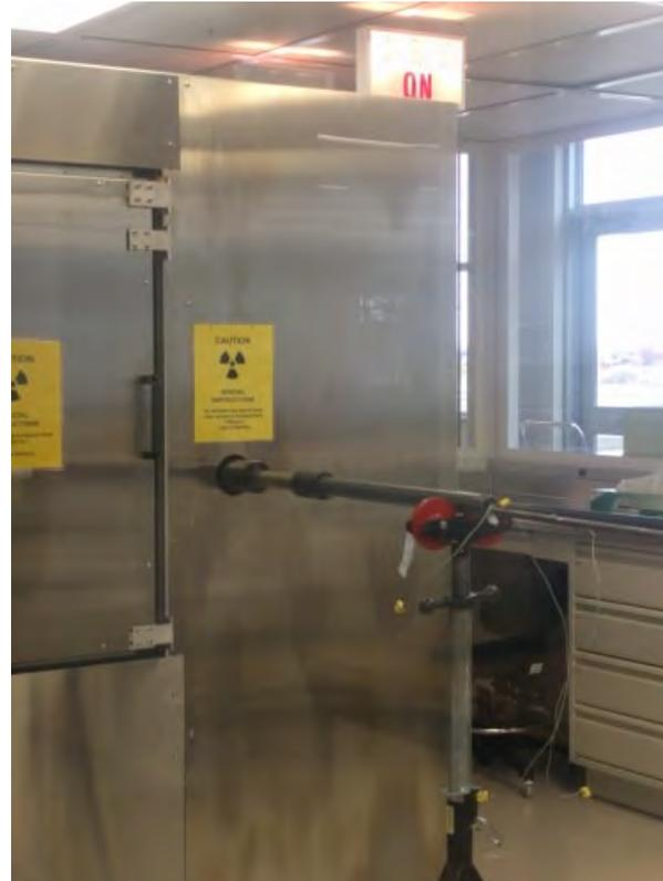
Specialized 3-D system with 1" through ports for long specimens
