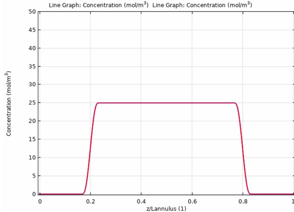
COMSOL Multiphysics<sup>®</sup> simulation of the evolution of a separation of two species with 0.25% difference in their electrophoretic mobilities in a 12-inch wide recycle CFE. Feed is continuously injected into the bottom center port and products are taken out of the chamber at the left and right offtake ports. Recycling allows the hold-up time to be increased until the two species are separated.
