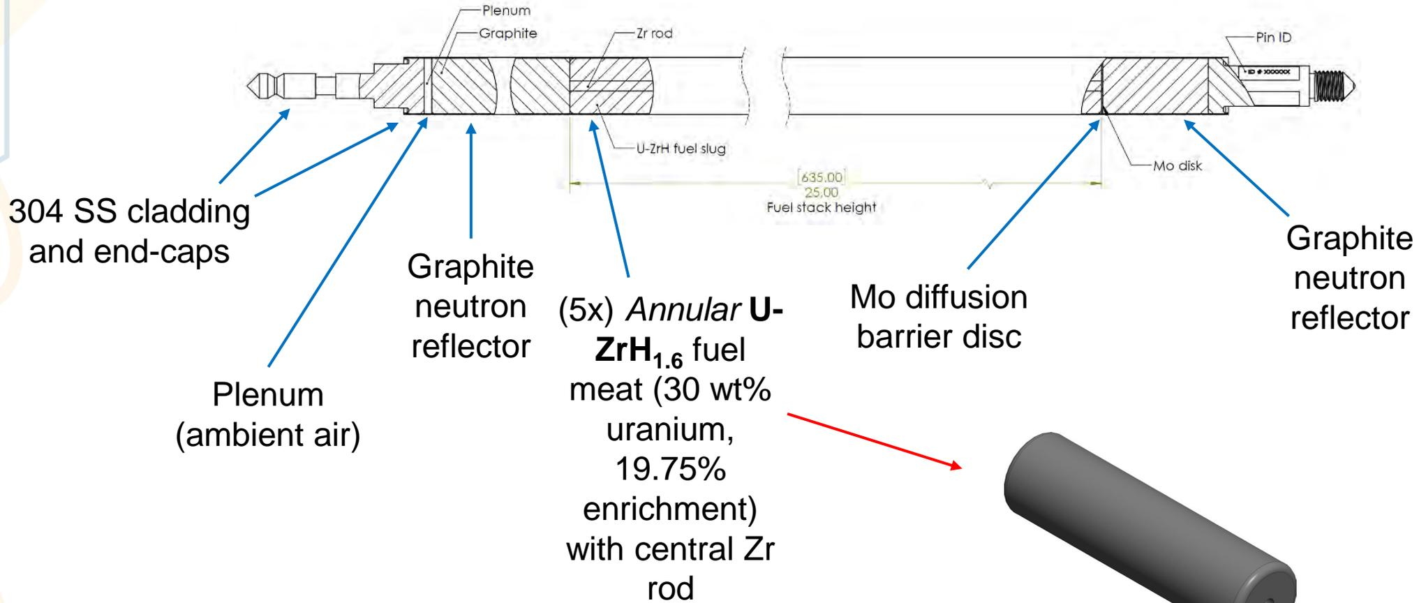
**U-ZrH<sub>x</sub> contains both the fuel (uranium) *and* neutron moderator (hydrogen) in one, reducing the size requirement of the reactor core to achieve the desired neutron energy spectrum**
