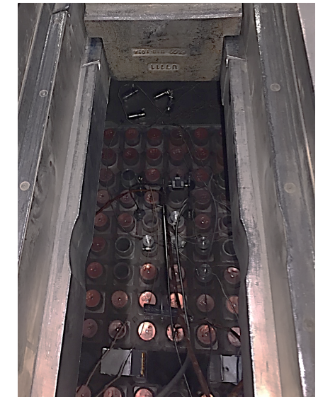
Top View of TREAT core with instruments inserted
