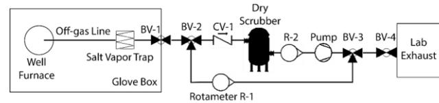
Multi-kilogram salt purification system diagram
