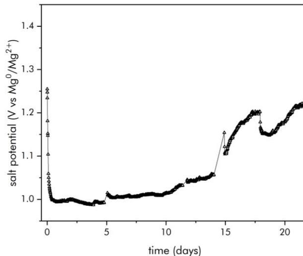
Salt potential vs. time during typical TCL experiment
