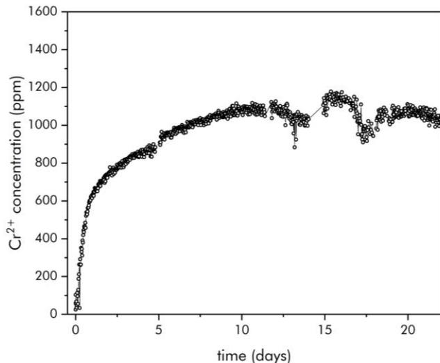
Cr<sup>2+</sup> concentration vs. time during typical TCL experiment
