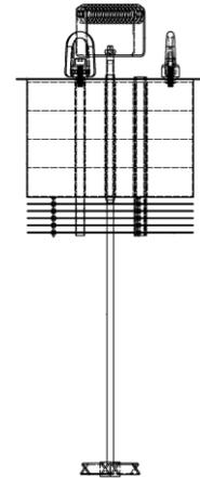
Heat shield assembly for actively stirred purification process with reactive metal contacting
