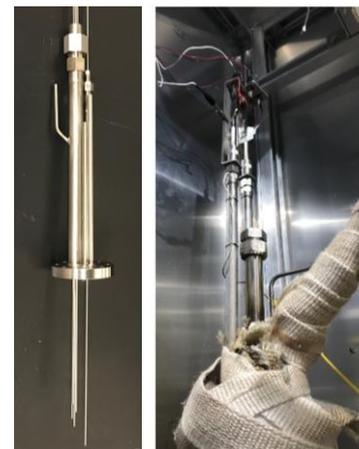
Typical multielectrode array sensor
