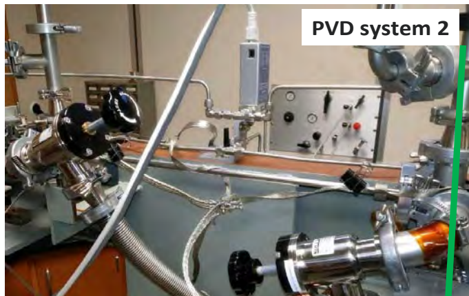
Internal surface coating facility (metal/alloy layer)
