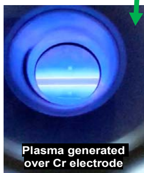
Internal surface coating facility (metal/alloy layer)
