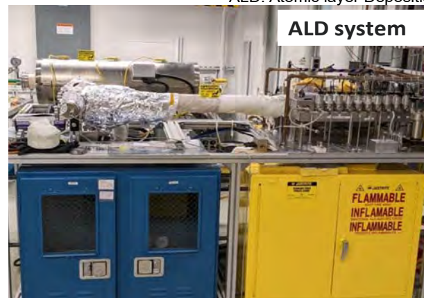
Internal/External surface coating facility (Ceramic layer)
