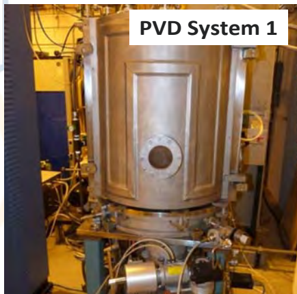
External surface coating facility (metal/alloy layer)
