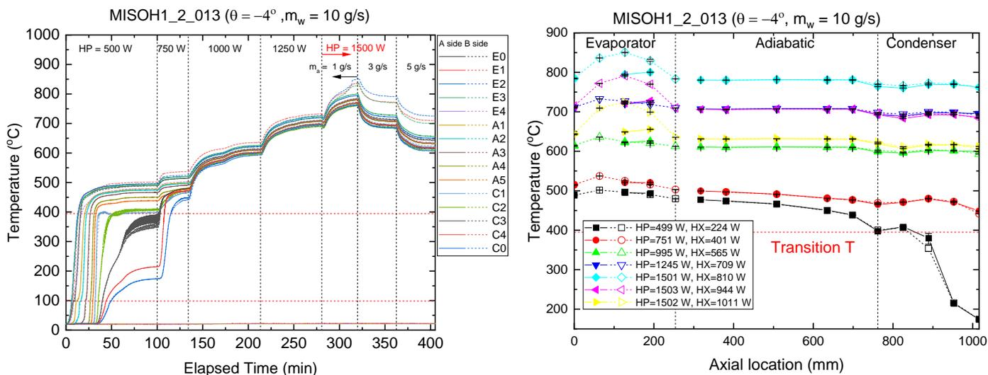
**MISOH1\_2\_013:** Comparing the steady-state temperature profile between pink and dark blue and between yellow and green. B side at evaporator was overheated under high heat transport rate with the same sodium vapor temperature. It is because more sodium is needed to support such a high heat transport rate so insufficient liquid sodium at B side lead to overheat
