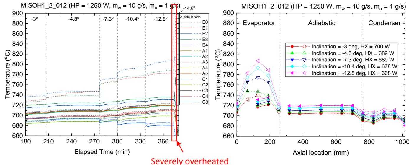
**MISOH1\_2\_012:** As the input power  $\leq 1000$  W, the heat pipe can be operated under -15 deg, but the temperature becomes not isothermal (overheated at the B side of the evaporator and subcooled at the A side of condenser end). On the other hand, severe overheat occurred as the input power approaches 1250 W under -14.6 deg
