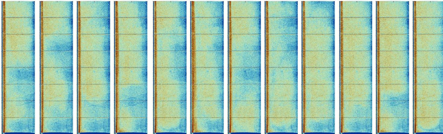
The sodium vapor was mostly generated from the B-side during the transient process, which matches with the temperature readings (B side temperature was higher than A side in the evaporator)
