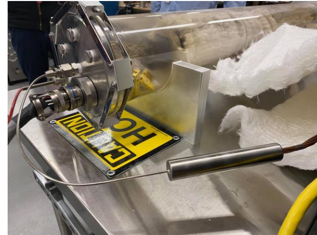
Thermocouple installed in SPHERE
