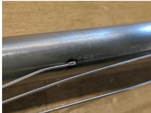
Thermocouple weld mockup
