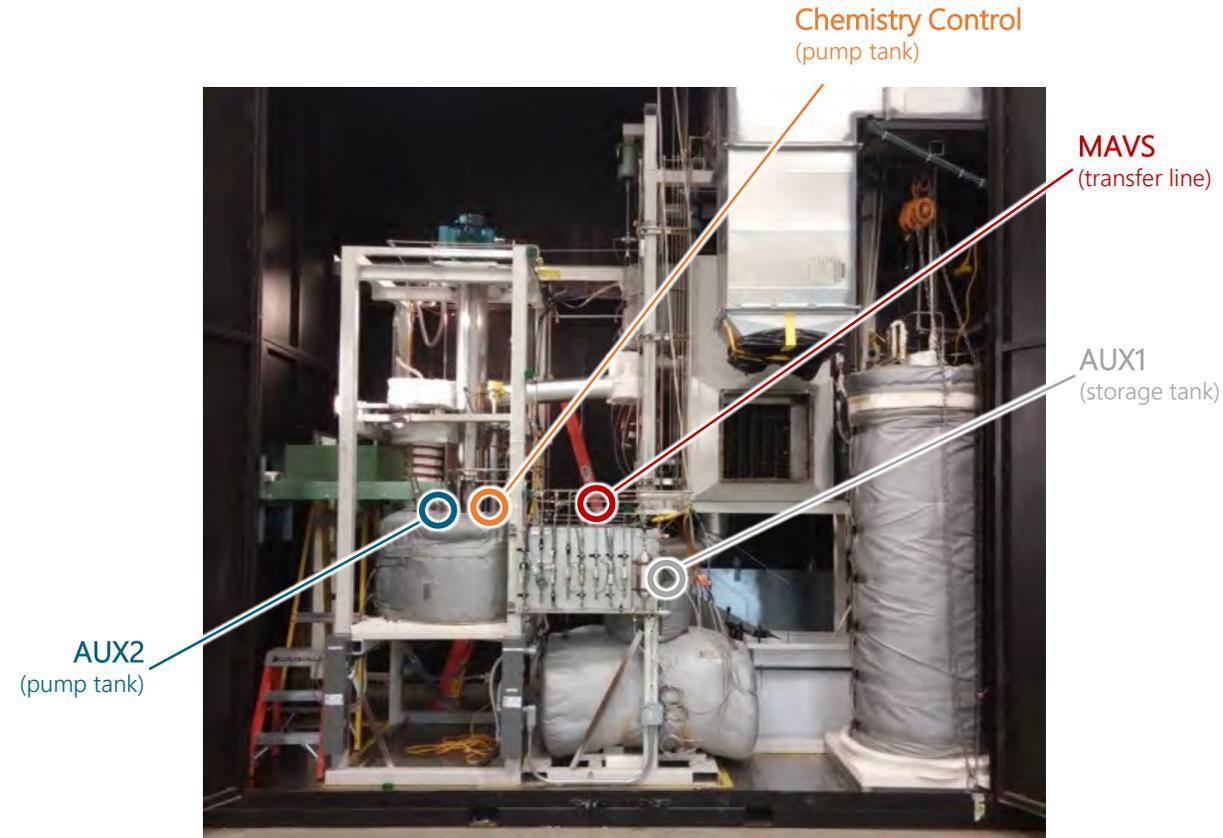
*Liquid Salt Test Loop at ORNL*
