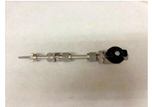
System designed at ANL to perform in situ impurity additions to molten FLiNaK and electrochemical measurements
