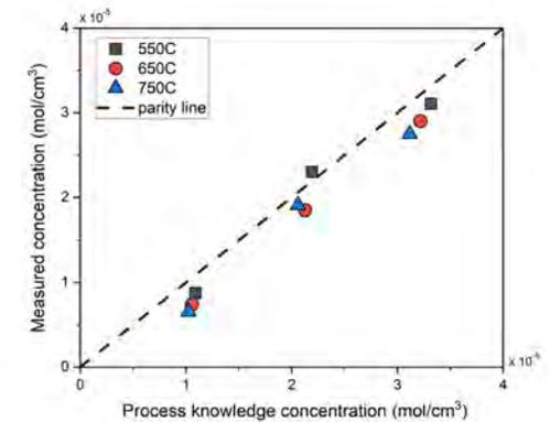
Raw Zr<sup>4+</sup>/Zr<sup>0</sup> LSVs (top left); Potentiometric relationship for Zr<sup>4+</sup>/Zr<sup>0</sup> (top right); Diffusion coefficients for Zr<sup>4+</sup> (bottom left); Measurements of Zr<sup>4+</sup> concentration (bottom right)
