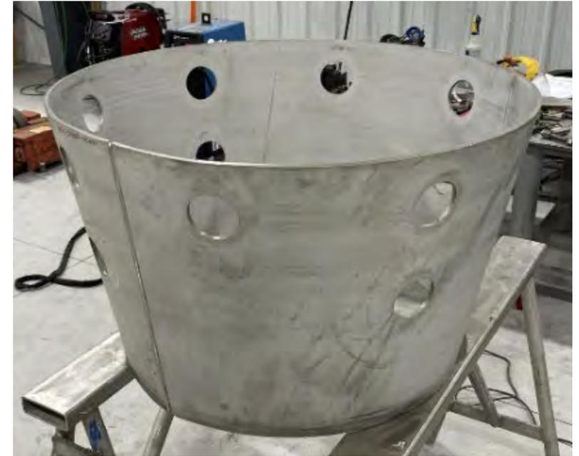
*Guard Vessel Tapered Wall*
