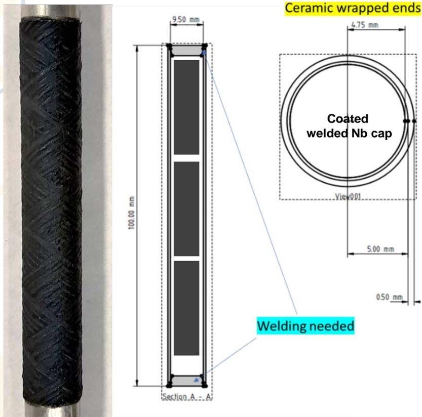
Schematic of the final AMM prototype containing  $\text{YH}_{2-x}$  pellets (3x)
