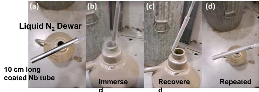
Despite extreme low temperatures & stresses of rapid contraction/ expansion, Cr<sub>x</sub>Al<sub>y</sub>/Al<sub>2</sub>O<sub>3</sub> coating remain adherent to Nb substrate.
