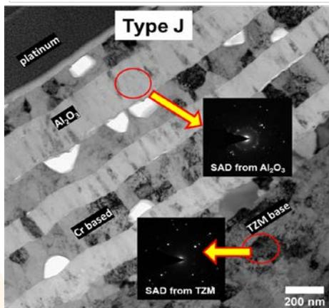
TEM image taken from multilayer cross section after exposure to pure H<sub>2</sub> (100 Kpa) at 700 °C
