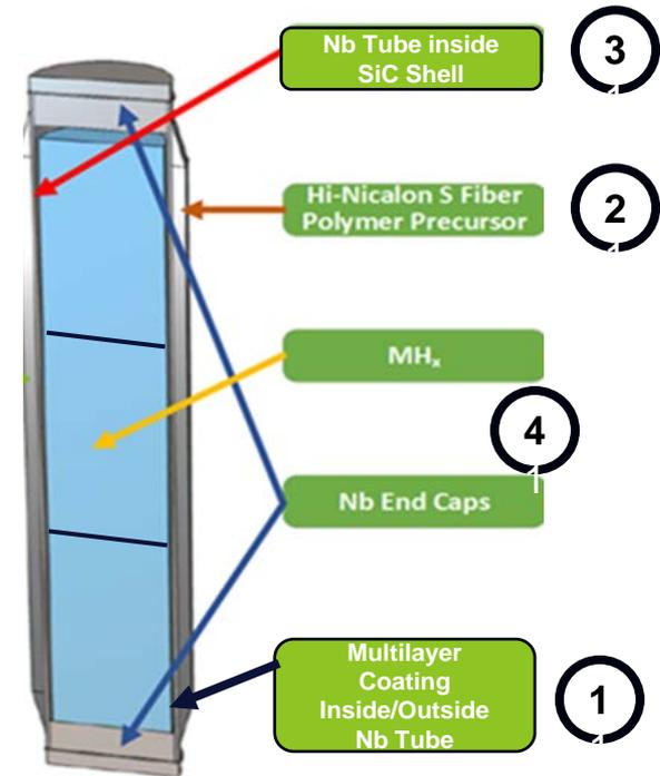
Schematic of the AMM Cross section , showing the metal hydride pellet within Nb liner, and enclosed by two Nb caps, welded on both ends.
