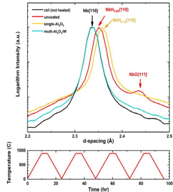
No hydridation or oxidation of the Nb substrate with coating present, measured after performing thermal cycling at 900 °C
