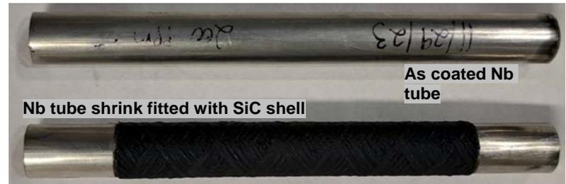
SiC-coated Nb liners of various lengths were manufactured
