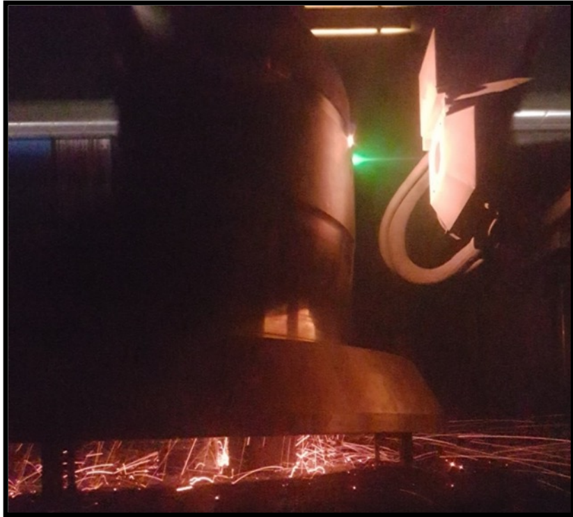
Circumferential Welds Completed in < 60 minutes
