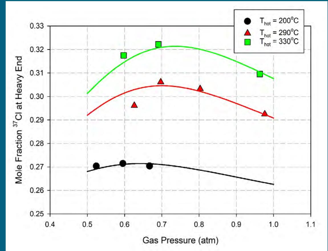
Measured and modeled pressure dependence of isotope separation for multiple temperatures.
