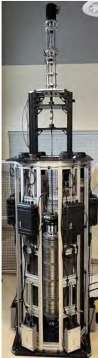
MARVEL Control Drum Prototype in ASI Double Delta Platform
